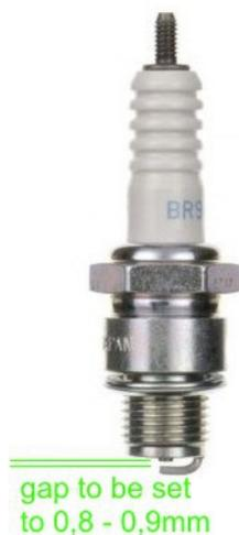
A too wide gap resulting in lack of strength of the spark or interruptions. A too narrow gap resulting in inexact sparks and possible additional sparks at wrong times. Use an accurate feeler gauge to receive a correct measurement!
