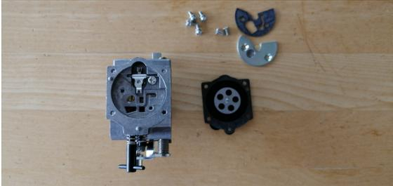
remove the paper gasket also. Use a small sharp screw driver to get it out as it may stick, but use precaution not to damage it!
