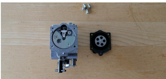
open cover by removing the 4 screws, put cover and gasket incl. lever plate aside. You need to slide out the nipple from the fork of the lever to be able to remove the plate. Use precaution here not to bend the lever or damage / misshape the lever plate!
