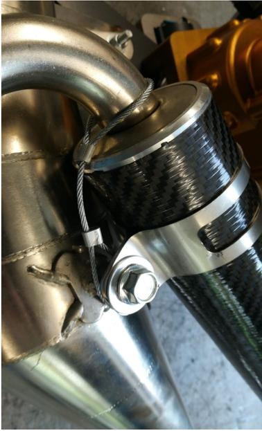
finish the wire loops by using press sleeves to fit the wire
