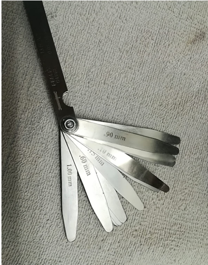
feeler gauge tool to correctly measure ring gap
