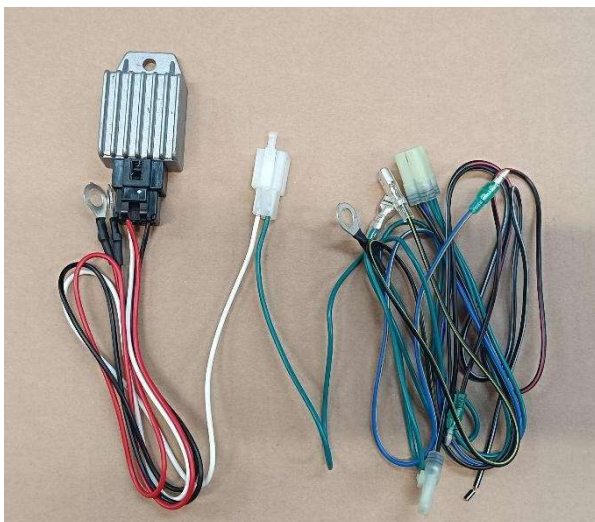
Fig 10a. Wiring Harness for battery charging
